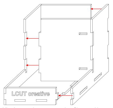
Join the 2 assemblies from previous page together. Clamp and leave to dry.
