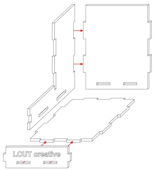
Start by joining the floor, front element, one side element, and back element together.
